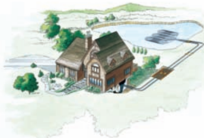
Pond Loops: Coils of pipe are fabricated and sunk to the bottom of the pond.
