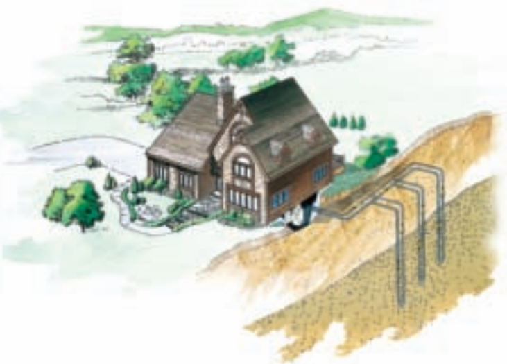
Vertical Loops: Used where land area is limited or soil conditions prohibit horizontal loops. Installed using a drilling rig.
