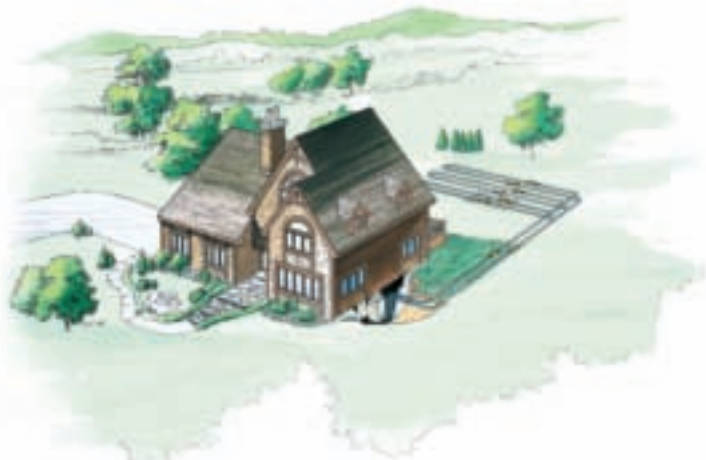
Horizontal Loops: Used on larger lots. Installed using a backhoe or trencher.
